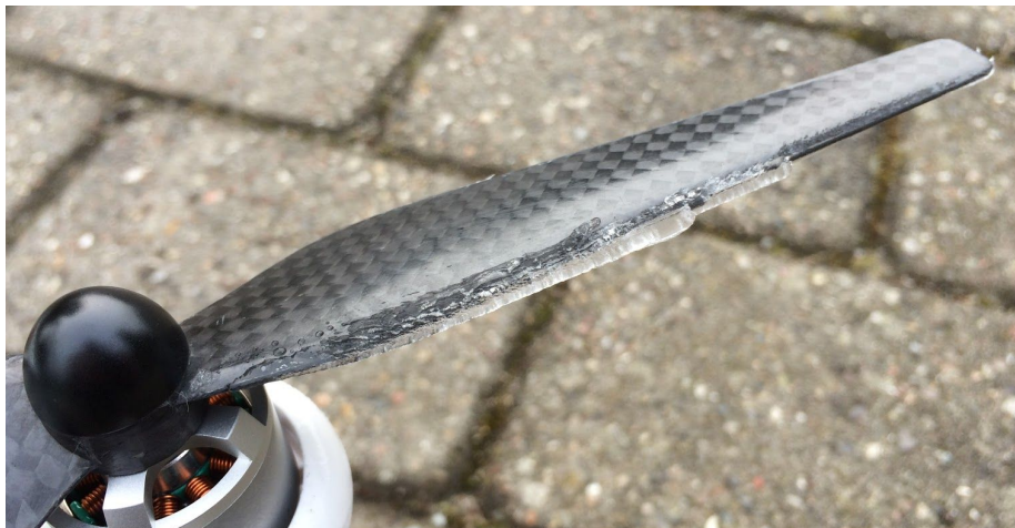
Figure 1: Clear ice protrusions on the propeller of a DJI Phantom 3 Advanced UAV disrupting the airflow and thus reducing the resulting lift. The image was taken after a 10 minutes flight in Odense Municipality, Denmark, March 12 2016 at 08:50 where the surface temperature was 0.8 [°C] and the dewpoint temperature -0.97 [°C], according to the historical data provided by IBM, thus resulting in a temperature-dew point spread of 1.77 [°C] and icing risk.
